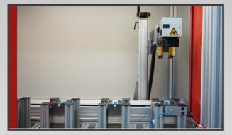
We create **multi-stock solutions** equipped with a **pick and place** system for loading/unloading the plate.
