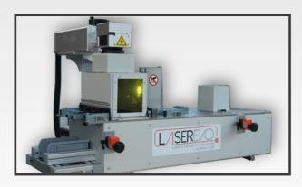
The benchtop **Tag-feeder solution**, equipped with an adjustable stock, allows you to mark plates of different sizes.
